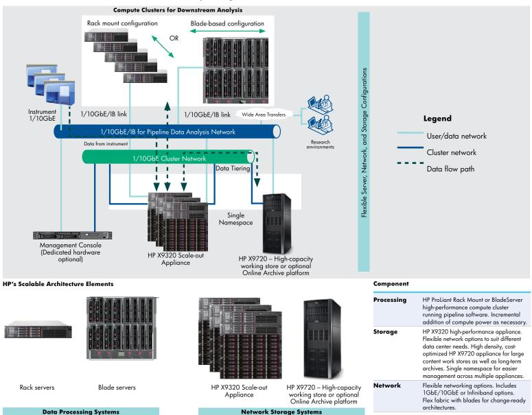
Figure 2. A network configuration example that implements the workflow illustrated in Figure 1. Several HP X9320 scale-out network attached storage appliances serve as the main performance working store, with an HP X9720 providing additional working store as well as archive within a single namespace over multiple data tiers. Depending on performance requirements, data processing and file system cluster networks can be 1 or 10 gigabit, or Infiniband networks.
