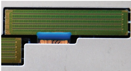
Figure 5 Detail of an HP Thermal Inkjet die
