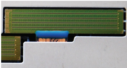
Figure 5 Detail of an HP Thermal Inkjet die
