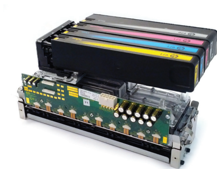
Figure 3 Pagewide writing engine assembly
