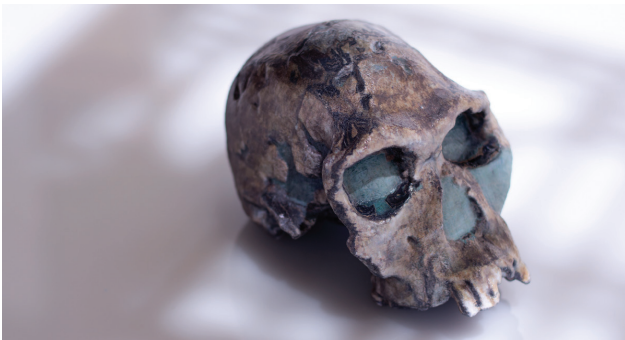
Archeology model 18.6in3 (304cm3) in size 3D printed from paper in full colour on an Mcor IRIS 3D printer and cost just $13.06 (€10.05).
